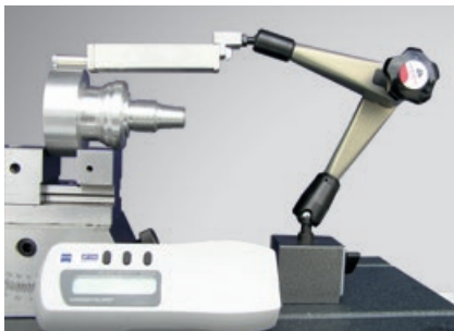
Magnetic column with ball joints Flexible magnetic columns with two ball joints and one swivel joint
