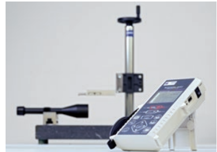
SURFCOM FLEX Compact control and analysis unit with integrated printer and Excel-based evaluation software
