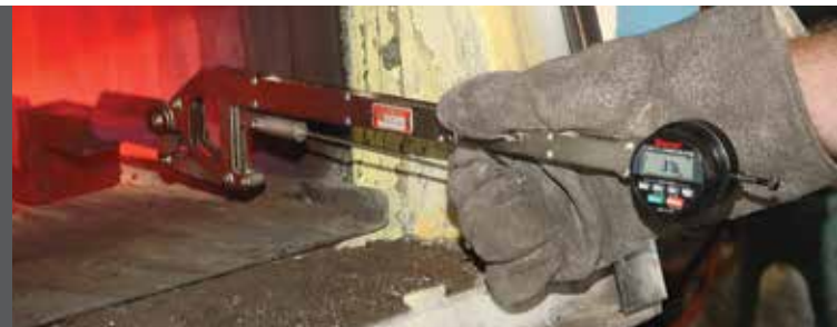
Variation on a theme: A large caliper with long reach for web thickness of train tracks hot or cold.
